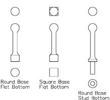
Length is From End of Ball to Flat Base (without stud). All Studs are 0.375" (9.53mm) Long
