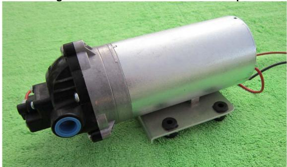
This is an industrial quality high pressure cold water pump designed to operate off of 12 volt battery systems. Adding a small motorcycle battery and this pump provides a safe and reliable alternative to injectors, axle pumps or steam driven pumps to add water to the boiler. Will self prime and can be ran dry without damage. Includes overpressure shut off switch.
